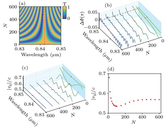
**Fig. 4.** (a) Transmittance spectra of structures of different  $N$ . (b) Phase differences  $\Delta\Phi$  between the top and the bottom surfaces in one unit cell with different  $N$ . The red dots and the dashed line indicate the zero phase difference at 0.842  $\mu\text{m}$ . (c) Group velocity of the structures with different  $N$ . The red dots show the group velocity at 0.842  $\mu\text{m}$ . (d) Group velocity at the degenerate point of the structures with different  $N$ .
