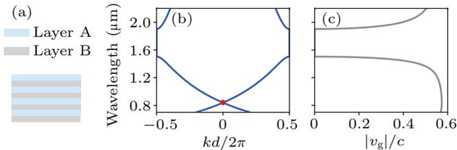
**Fig. 1.** (a) Schematic of the 1D periodic structures. (b) The photonic band structure. The red point marks a degenerate point. (c) The derived absolute group velocity.
